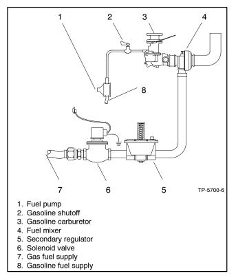
Figure 6-11 Combination Gas/Gasoline Fuel System
